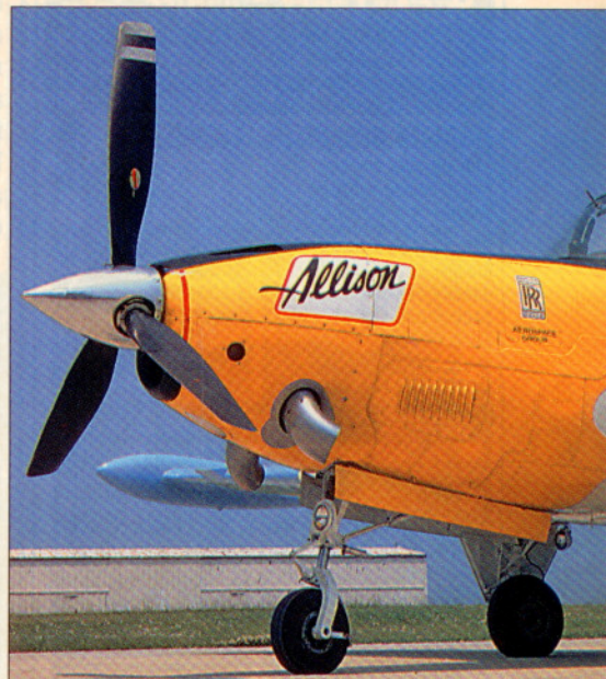
The Allison 250 has two more oil injector ports than standard, allowing 30 seconds of inverted flight.
