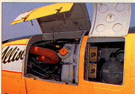
The Allison 250 has two more oil injector ports than standard, allowing 30 seconds of inverted flight.
