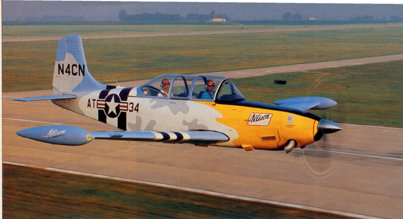
The vertical stabilizer was borrowed from a Travel Air, while the wing was built from Baron spars and Bonanza leading edges.
