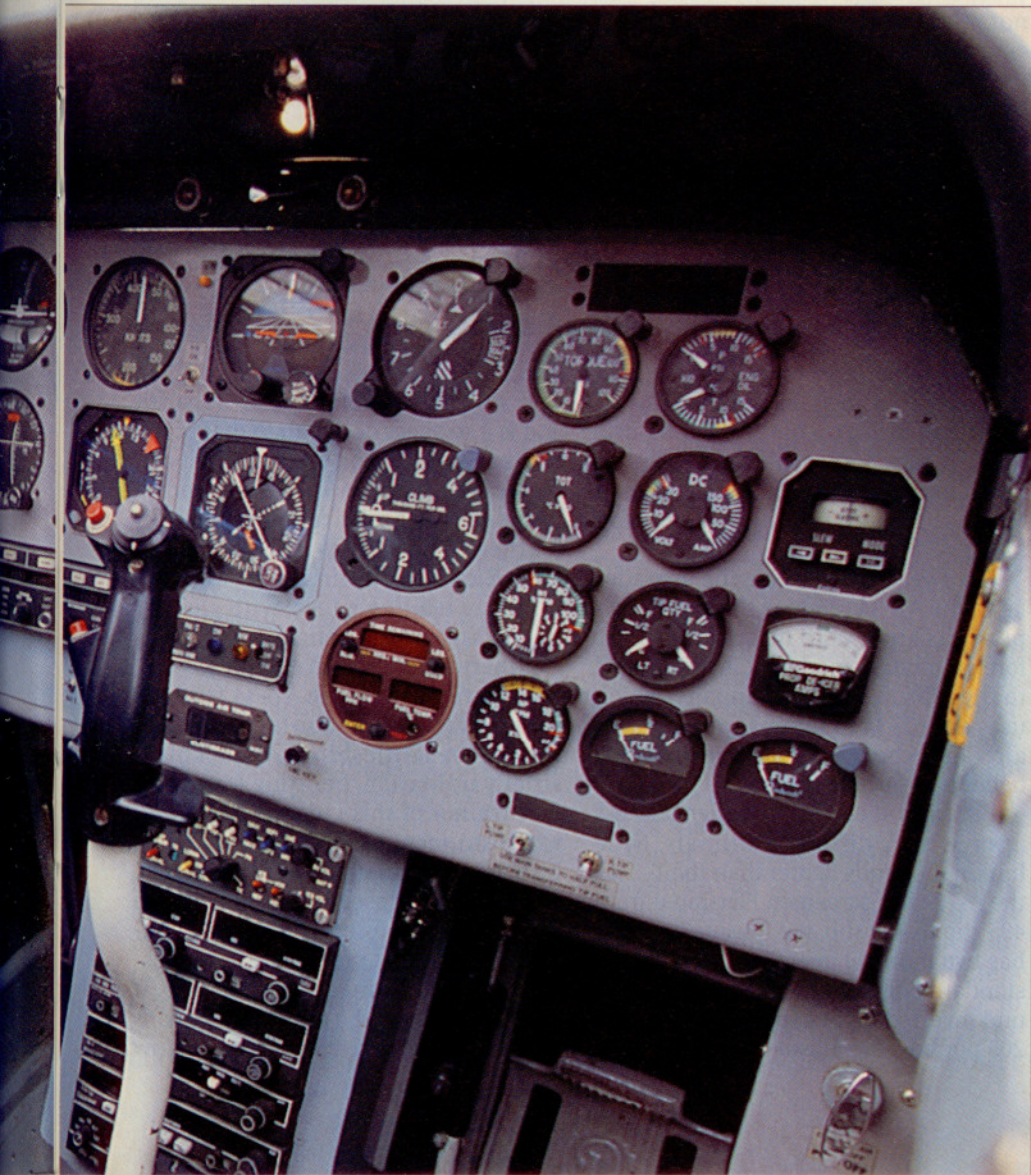
The fighter-style cockpit helped ease the transition to jets for military flight students. The Allison engine provides a climb rate of 2,800 feet per minute and a cruise speed of 170 knots.
